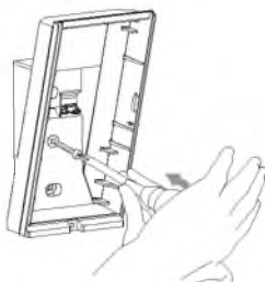
Knockout with 4 × 20 tapping screw (screwkit)
