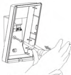
Knockout with 4×20 tapping screw (screwkit)
