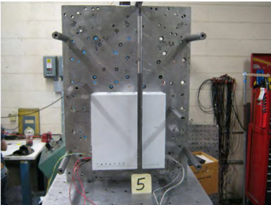
Shock test setup for EVO192 and ZX8
