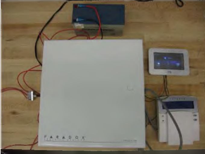
Photo 1: EVO192 Control Panel and TM40 Touch Screen – External View
