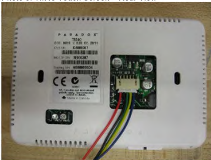
Photo 6: TM40 Touch Screen – Rear View
